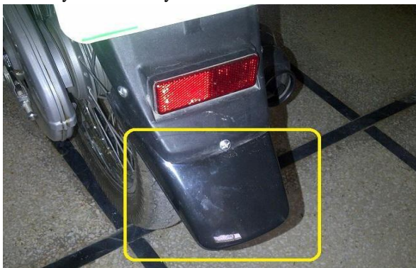
Fig.4.3 Mudguard with supplementary mudguard
