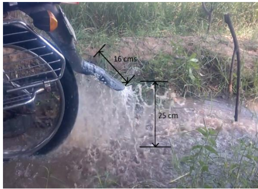
Fig.4.1 Experiments after additional mudguard
